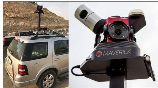
Figure 2. Maverick Mobile Mapping System Used for Pilot Project in Jordan
