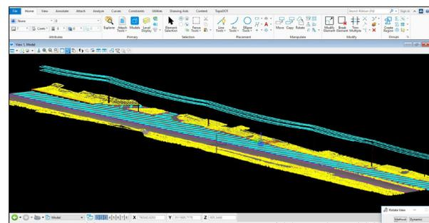
Figure 9. Road extracted features in CAD format
