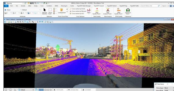
Figure 8. TopoDOT software point cloud overlaid over images
